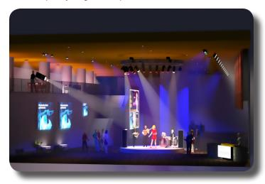
2) **Small school stage**. Proof of design that 6 fresnels and 4 ERS can light a stage with the correct products and placement. Previously this was all guesswork with 2D electrical plans.
